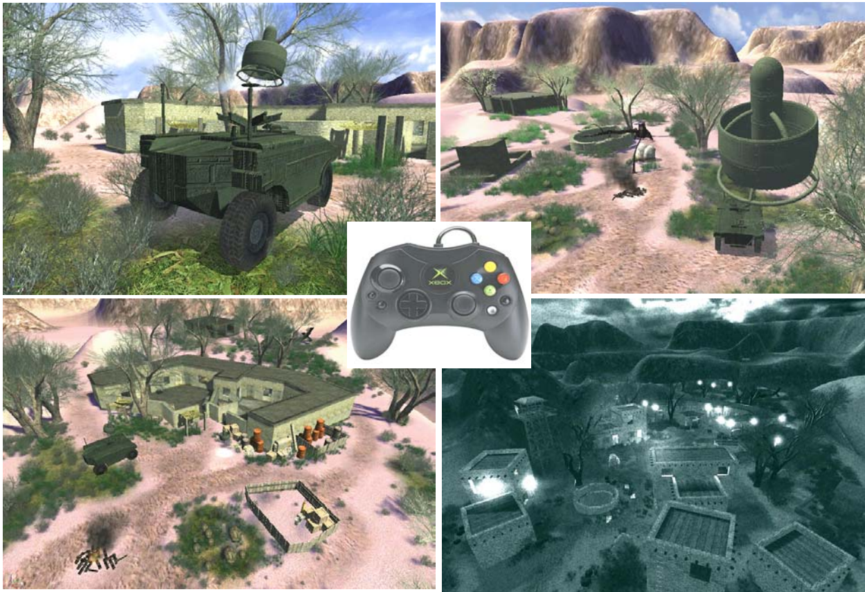
Figure 9: Various Views of the Alchemy 2 iSTAR UAV Demonstrator, Including Launch, Flight Over Insurgent Camp and Night Vision Capability (middle insert shows the Microsoft Xbox S controller used as one of the experimental UAV flight control options).
