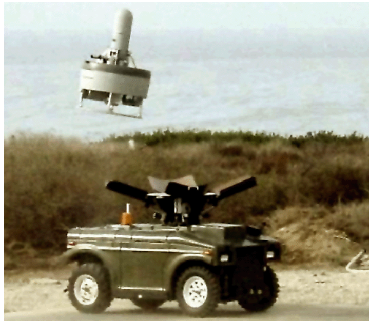
Figure 4: The SPAWAR MDARS-E Marsupial Vehicle Launching an Allied Aerospace iSTAR UAV (source: www.nosc.mil/robots/resources/marsupial/marsupial.html ).
